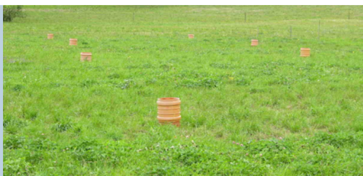
Figure 4. \text{N}_2\text{O} measurements in grasslands using the closed chamber technique.
