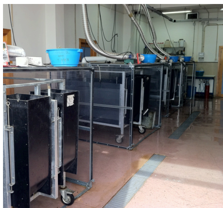
Figure 3. Set of 4 chambers to measure \text{CH}_4 and \text{CO}_2 production at EEZ, CSIC, Granada.
