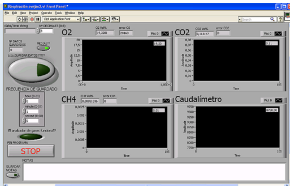
Figure 5. Panel of the LabVIEW program for monitoring gas analyser and the flow meter (appearing in Computers and Electronics in Agriculture).
