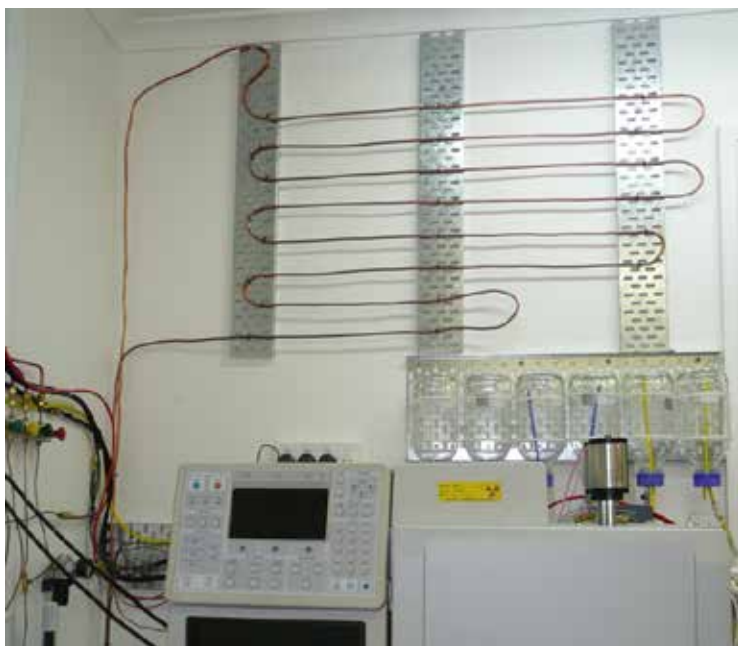
Figure 8.4: GC and copper tube array used to bring the temperature of the carrier gas to room temperature. At DPI Ellinbank, bottled gas is stored outside buildings for safety. In cold weather, it had been observed that the chromatogram baselines were unstable when the carrier gas was piped directly to the GC without temperature stabilisation.
