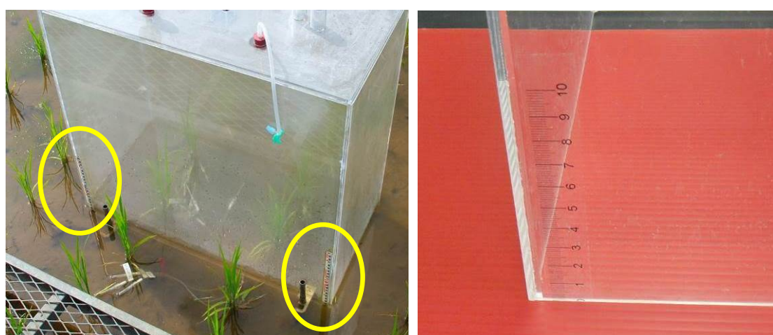
Figure 3.8. Examples of a ruler for reading the effective chamber height.
