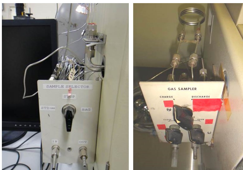
Figure 5.4. A gas sample loop and a manually switched injection valve.
