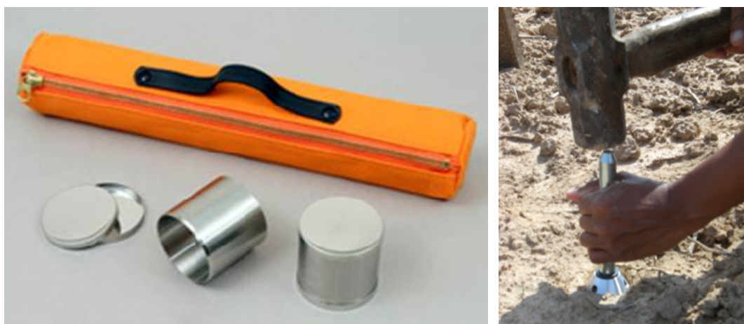
Figure 7.4. Stainless coring tubes (100 mL, left) and soil collection using a coring tube (right).
