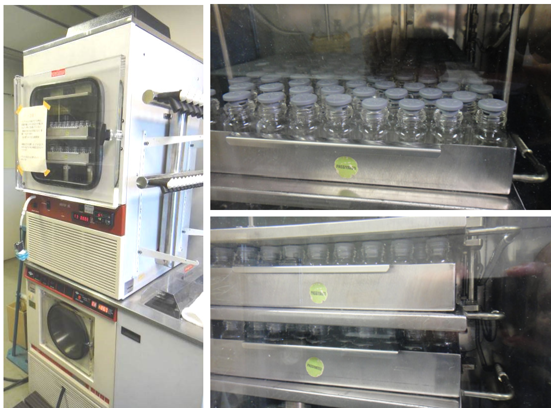
Figure 4.9. A vacuum freeze drier (left) with two trays for closing the vials with stoppers (right top and bottom).
