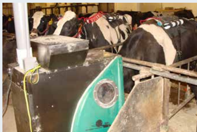
Measuring enteric methane emissions in US dairy cows.
