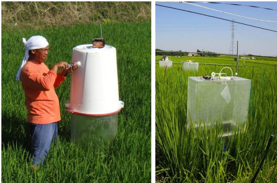
Figure 3.3. Examples of double-deck chambers.
