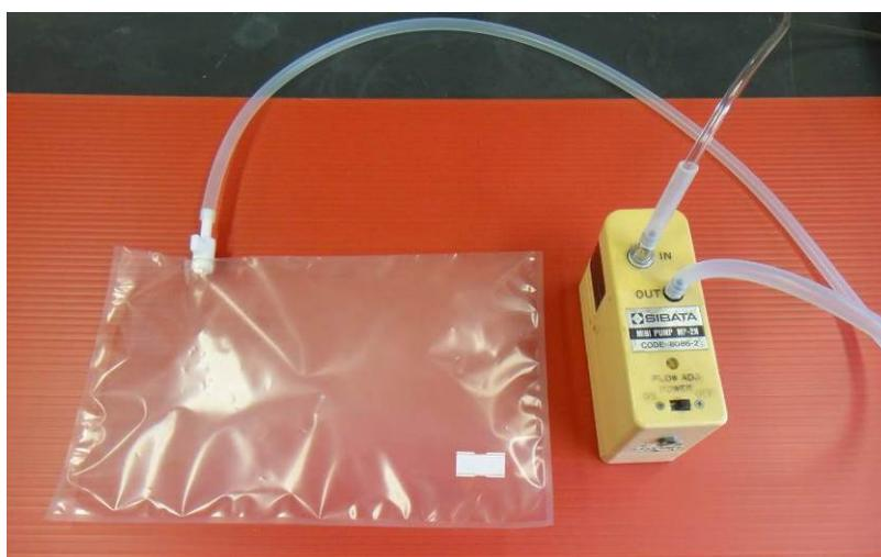
Figure 4.6. Gas being pumped into a plastic bag for storage.
