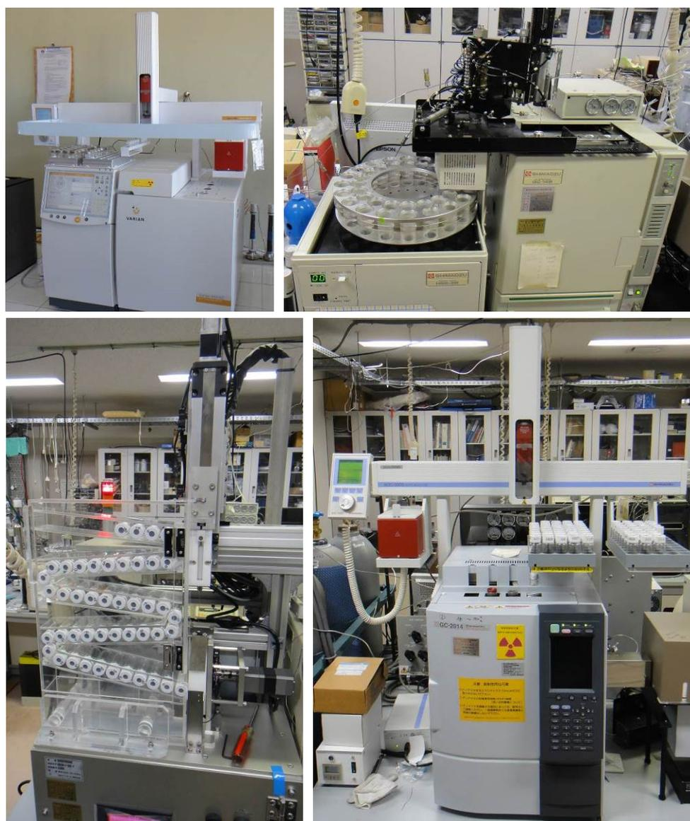
Figure 5.5. Examples of automated gas injection systems for glass vials.
