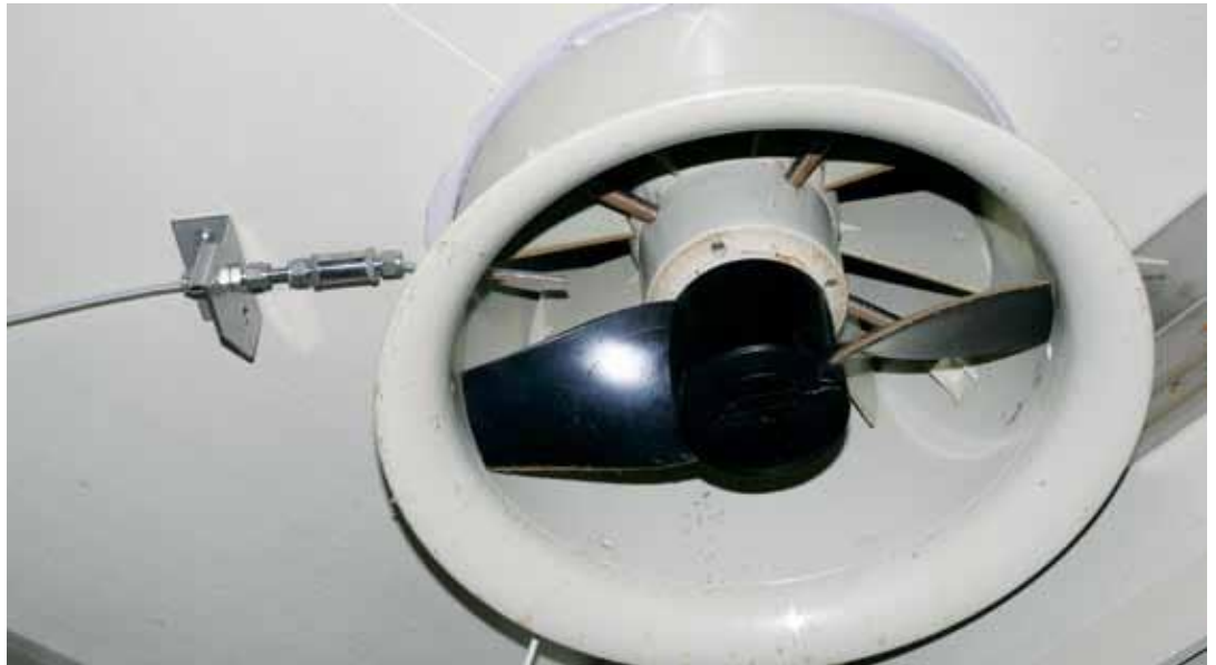
Plate 8: ATM-module with vortex damper (grey) and integrated impeller (black) . Gas sample point in ATM-module with sonic nozzle and 7 \mu\text{m} filter (left) .
