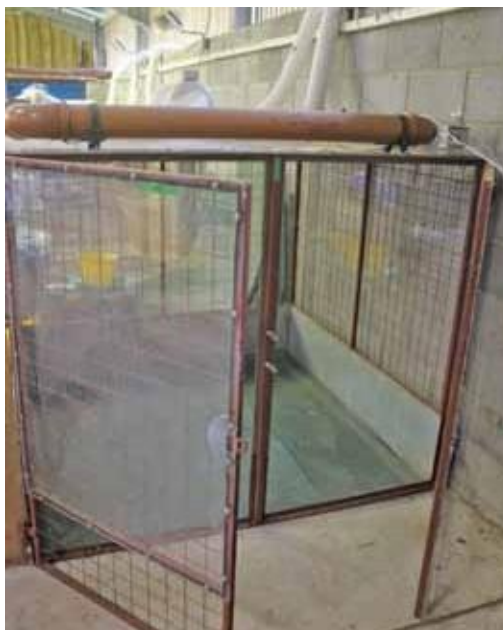
Plate 3: Front chambers at Aberystwyth University showing the gap at the bottom of the door to allow air to flow in.
