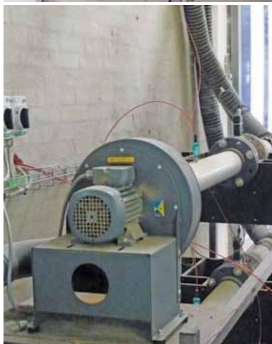
Left – Plate 9c: Motor and blower. Right – Plate 9d: Control box with individual motor controller.
