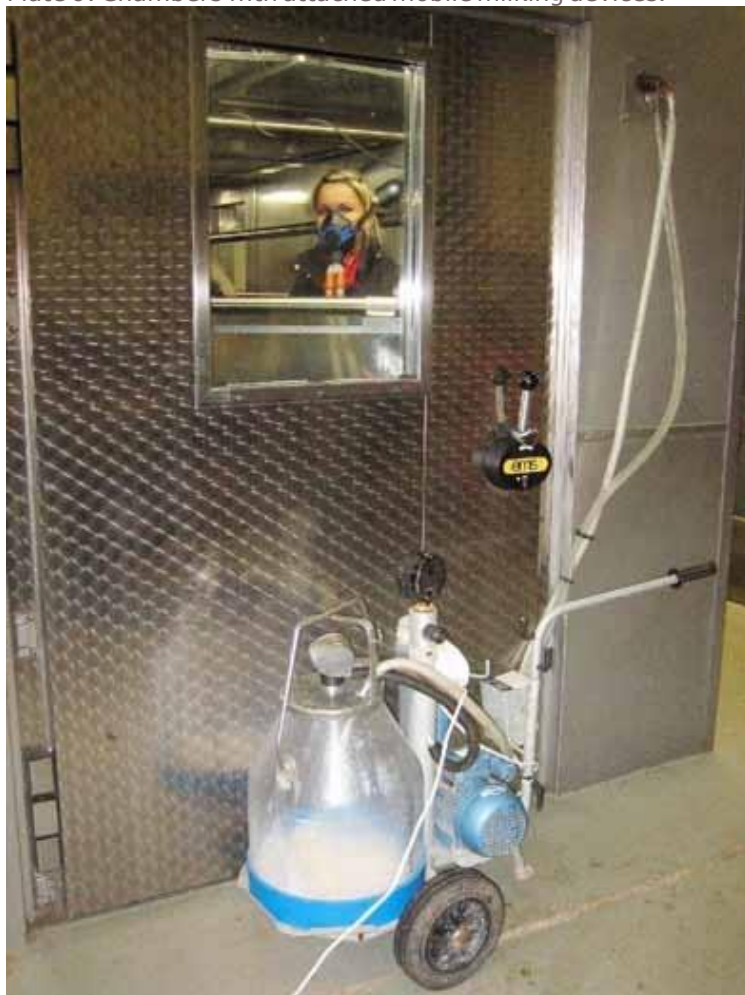
Plate 6: Chambers with attached mobile milking devices.
