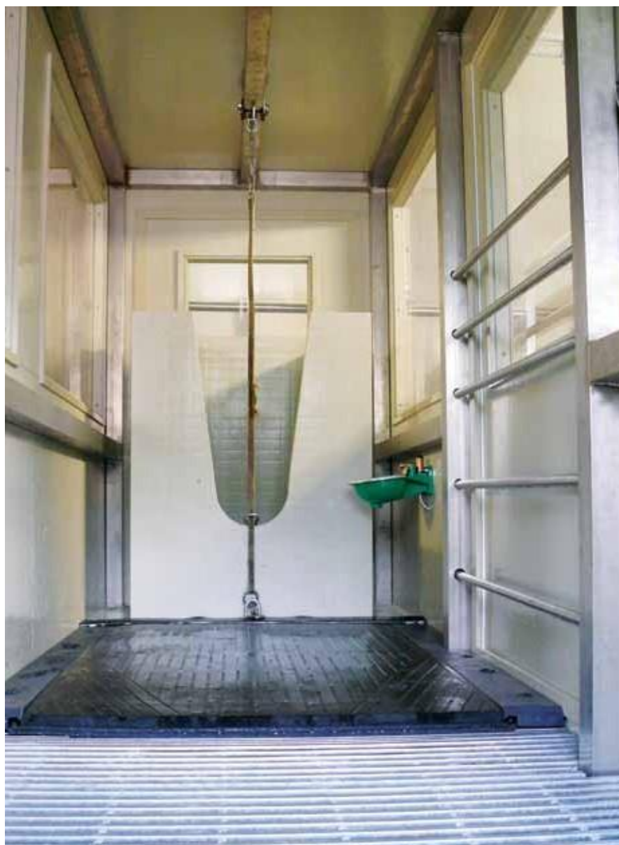
Plate 5: Inside view of a chamber made of polypropylene mounted on a stainless steel frame.
