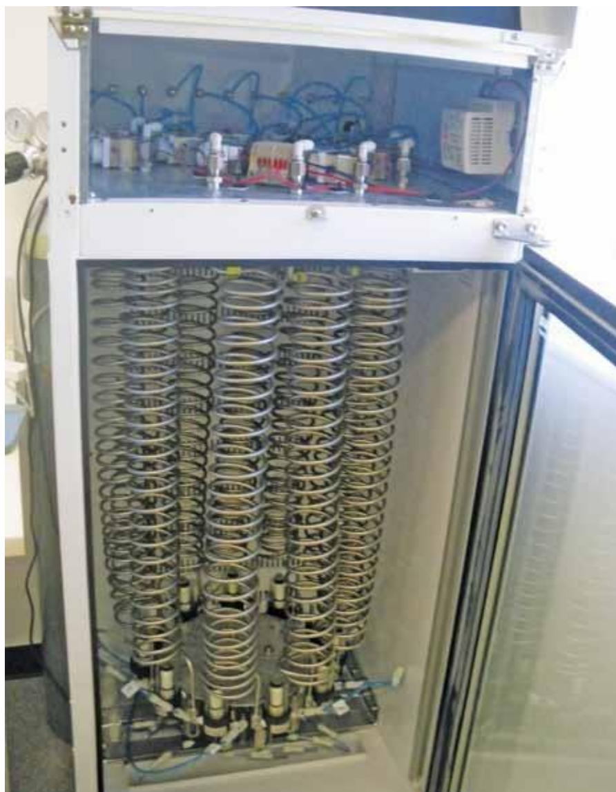
Plate 7: Sample drying system. Sample lines (10 sample + ambient) are drawn from the flow control manifold (Plate 6 above) at 1L/min by pumps mounted above the refrigerator (at top), which push the air through the refrigerated cooling coils which have autodrain of condensed moisture at the base.
