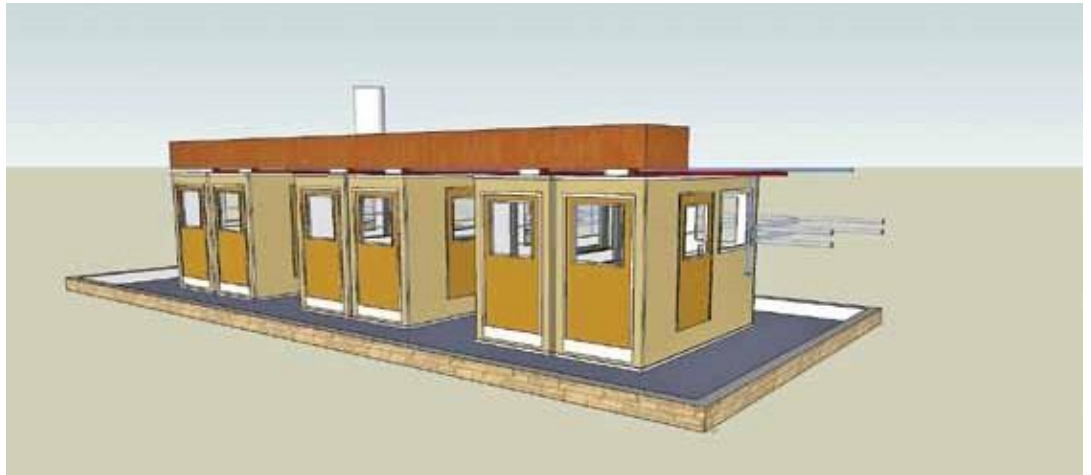
Plate 1: Drawing of ILVO's Ruminant Respiration Facility composed of six chambers.
