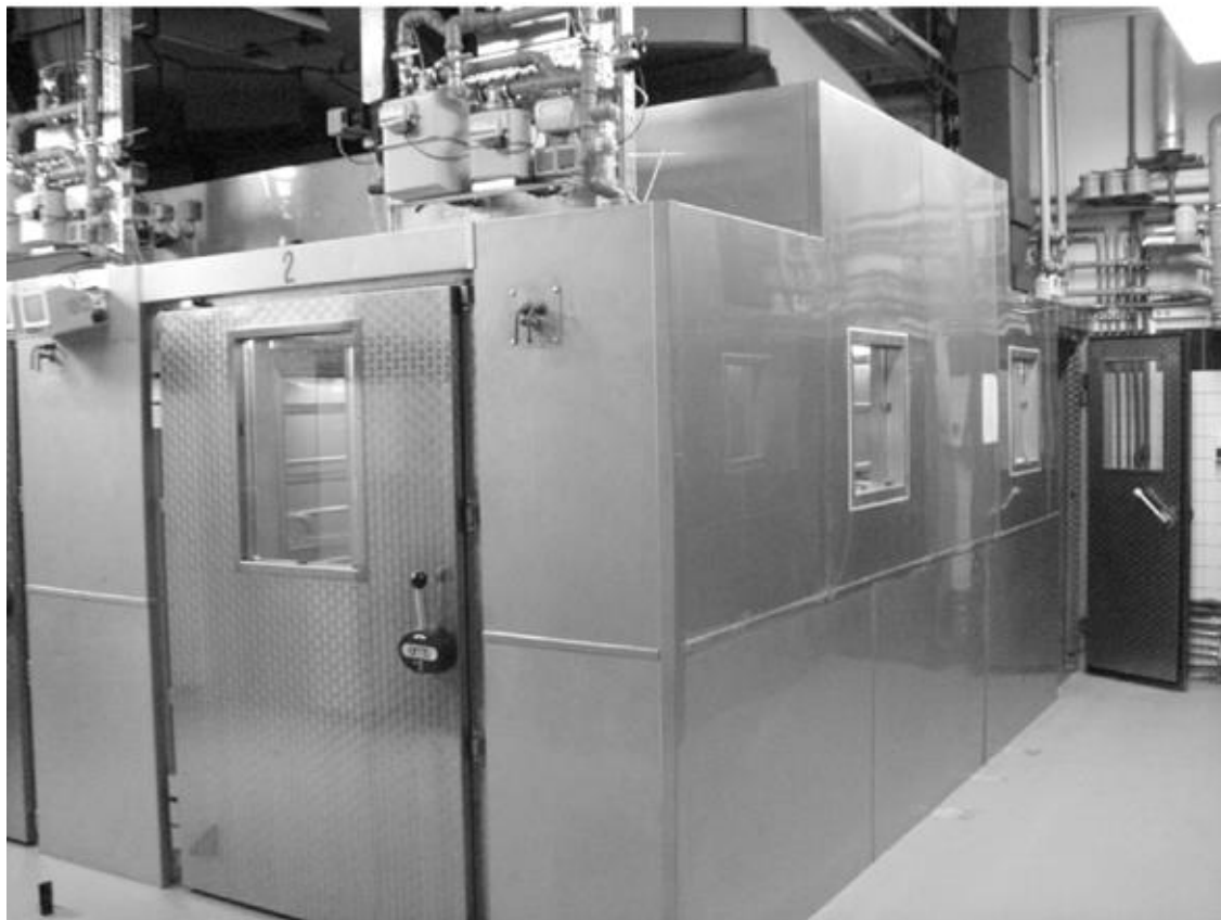
Plate 2: Respiration chamber for cattle with opened door to the airlock.
