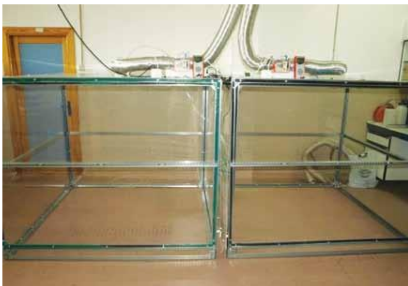
Plate 4: Front of two chambers at CSIC Granada showing the gap at the bottom of the door to allow air to flow in.
