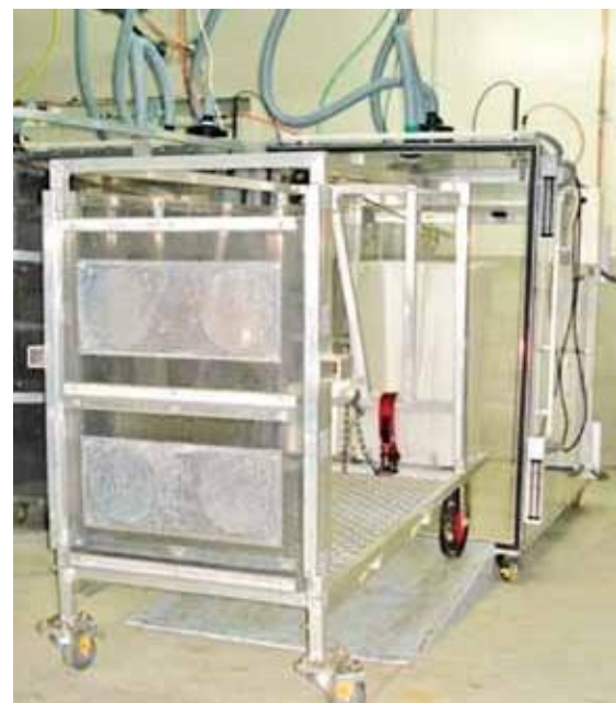
Plate 5: A ramp is used to wheel the sheep crate into the respiration chamber.
