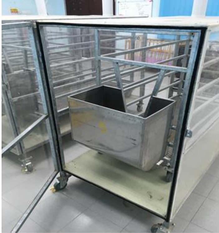
Plate 3: Front end of the chamber showing when door is opened, operator has free accessibility to feed trough and also shows strip of black fabric-lining to ensure no leakage of chamber air when operates under low flow rate.
