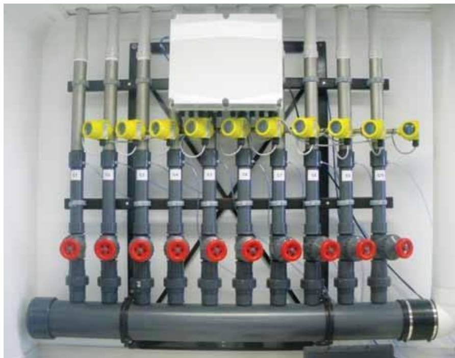
Plate 6: Flow measurement manifold featuring 10 mass flow meters with digital output and gate valves to control flow.
