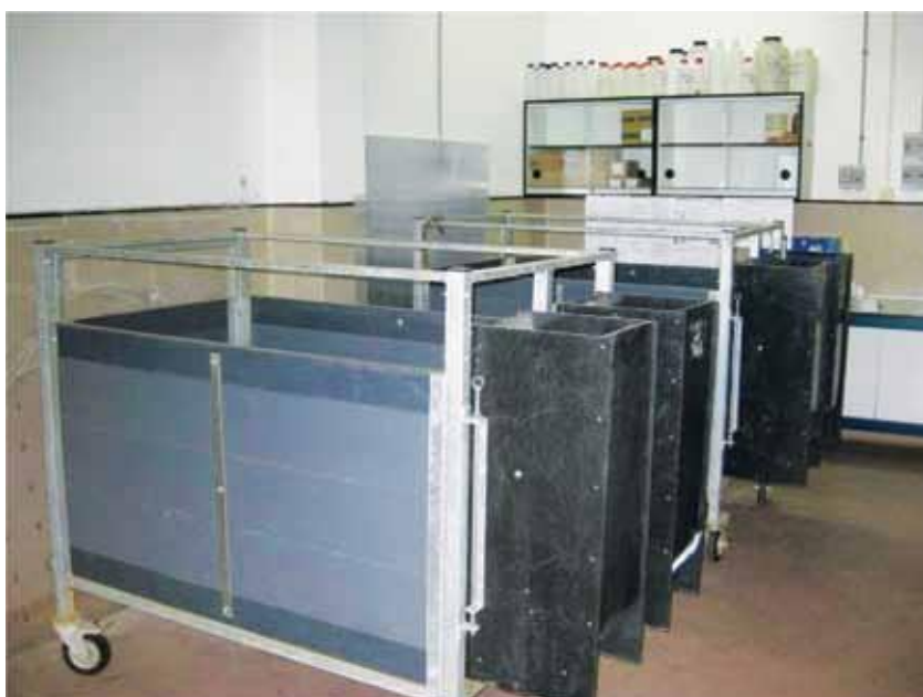
Plate 5: Mobile crates at CSIC to hold the animals during adaptation and in the respiration chamber.
