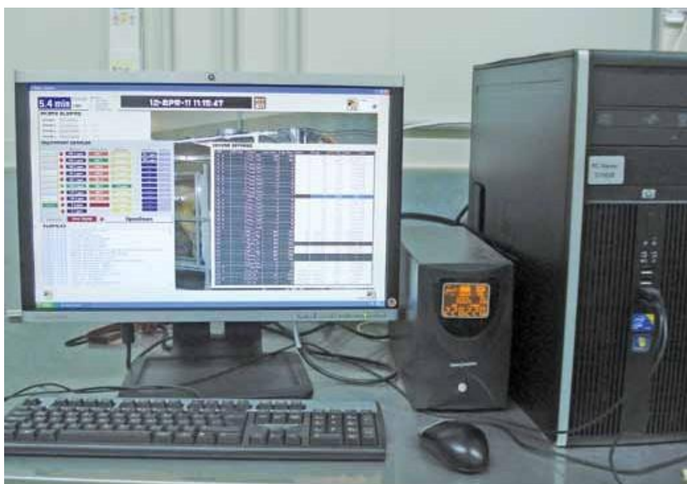
Plate 13: Computer (and power up system) with alarms set for abnormal environment conditions.
