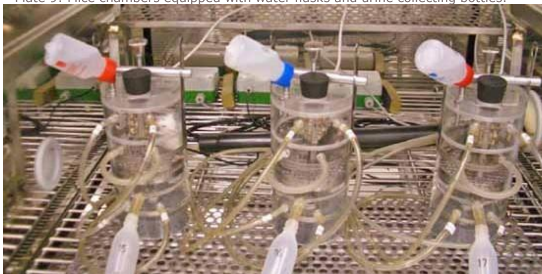
Plate 9: Mice chambers equipped with water flasks and urine collecting bottles.
