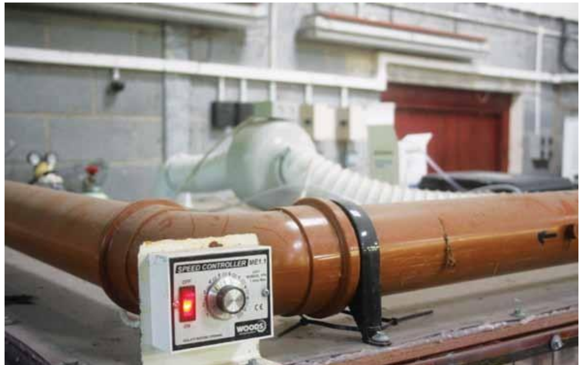
Plate 8: The variable fan speed controller and the inline fan positioned on the top of each chamber, at Aberystwyth University.
