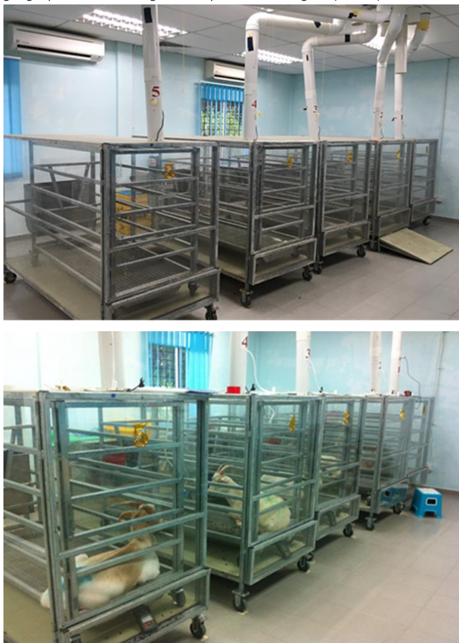
Plate 2: The five open circuit respiration chambers arranged in a row (top) and an on-going experiment measuring methane production from goats (bottom)
