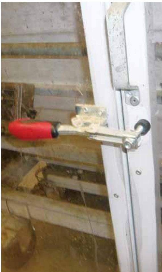
Plate 7: Lock clamp used to ensure that the front and back doors are closed, and a picture of the front door.
