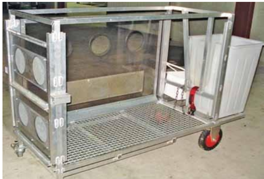
Plate 5: A ramp is used to wheel the sheep crate into the respiration chamber.
