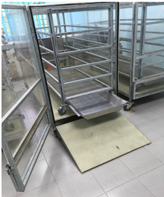
Plate 4: Views from rear end of the chamber showing the waste collection tray, small window at the lower section of the rear door which when opened allows accessibility to the waste collection tray without need to open the whole rear door (left). Roller-wheels are attached to the chamber and animal crate to allow them to be moved easily when necessary.
