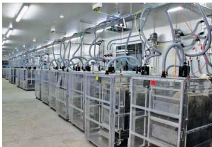
Plate 1: The sheep respiration facility comprises 24 chambers housed in a dedicated building.
