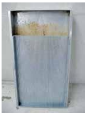
Plate 6: The mesh faecal collection tray fits on top of the stainless steel urine collection tray and both slide underneath the modified metabolism crate. Exchange of trays during cleaning is facilitated by a use of a trolley and waste bin.
