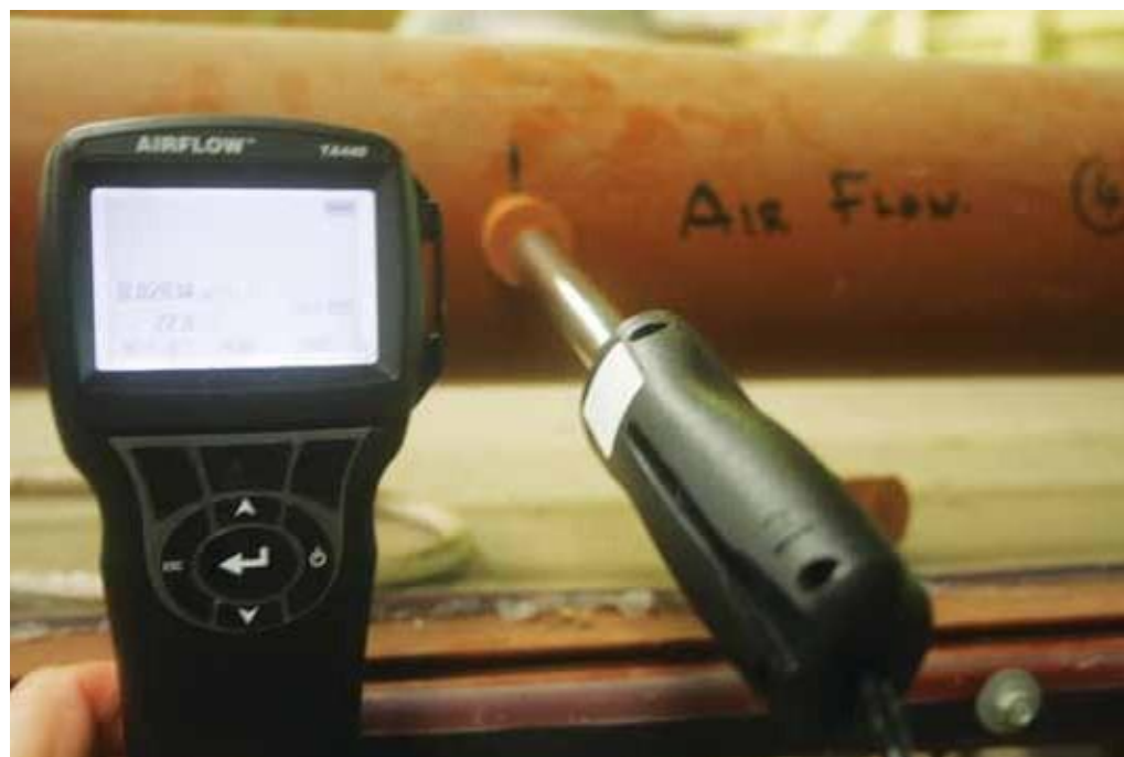
Plate 6: Top of the chamber at Aberystwyth University showing hand held flow meter inserted into the exhaust pipe.
