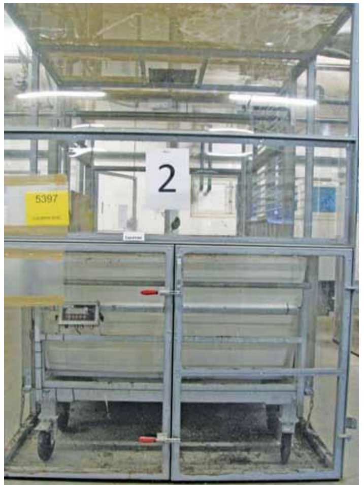
Plate 7: Lock clamp used to ensure that the front and back doors are closed, and a picture of the front door.
