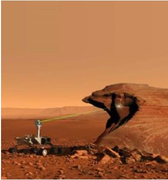
Figure 1: Nasa`s rover curiosity illustration that used a miniaturized LIBS spectrometer to soil and rock analysis in Mars (a) a LIBS typical spectrum of a solid material (b).
