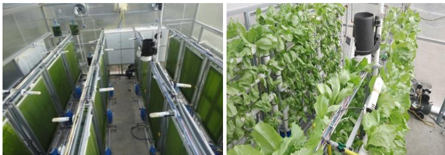
Figure 4: On the left, laminar photobioreactors for the production of microalgae and on the right, lettuce plants cultivated with microalgae.
