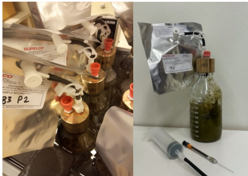
Figure 1. Modified in vitro system for determination of long term methane emissions from feces (nine weeks incubation).
