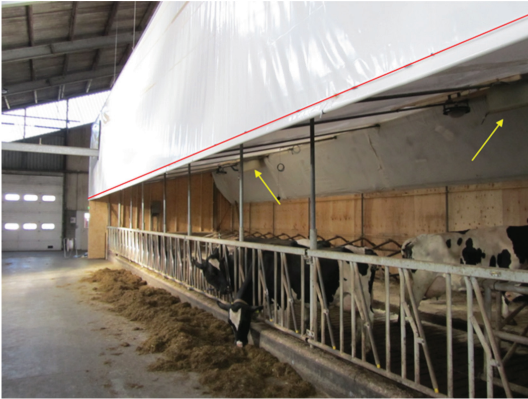
Figure 2. Overview of 1 of the 4 barn units, with curtain in lifted position. Red line indicates the sampling line for incoming air concentrations. The yellow arrows indicate the 2 ventilators including sampling lines for outgoing air concentrations.
