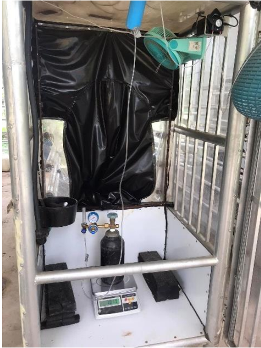
Photo of gas recovery in action
