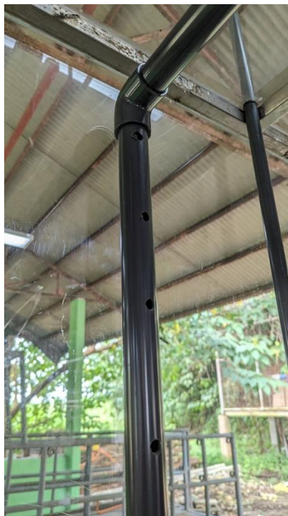
f. Vertical 1-inch pipes with holes for the entry of air to be analyzed
