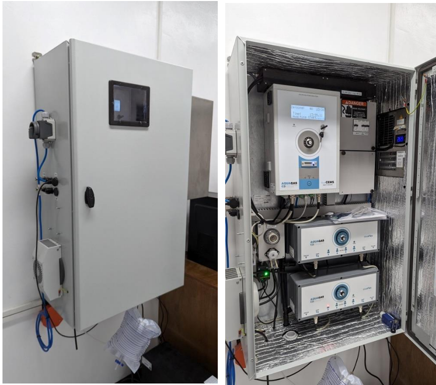
l. The gas analyzer with multiplexer used at DTRI - UPLB
