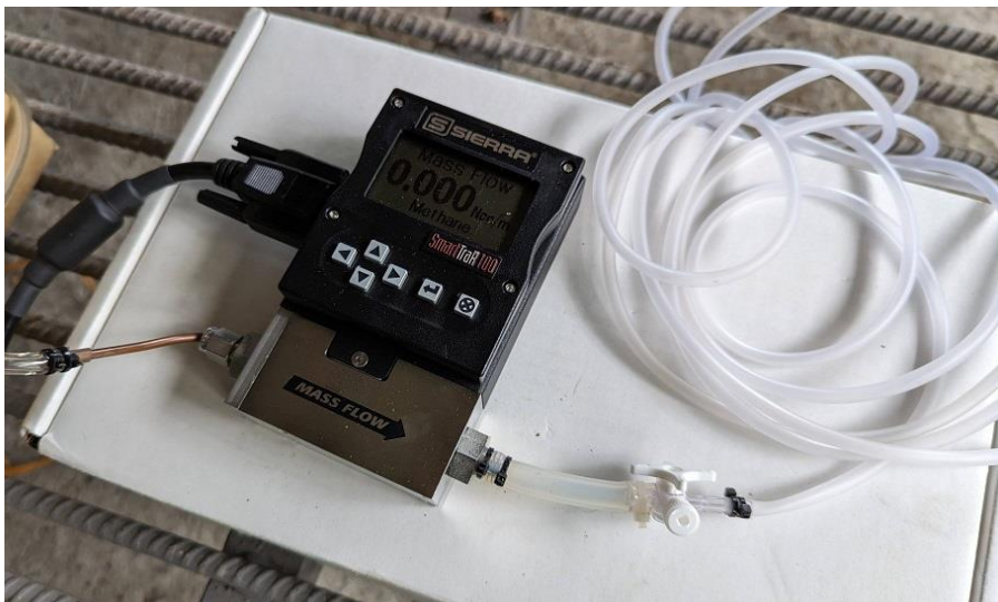
m. The mass flow controller used to infuse a known and steady amount of gas into the system
