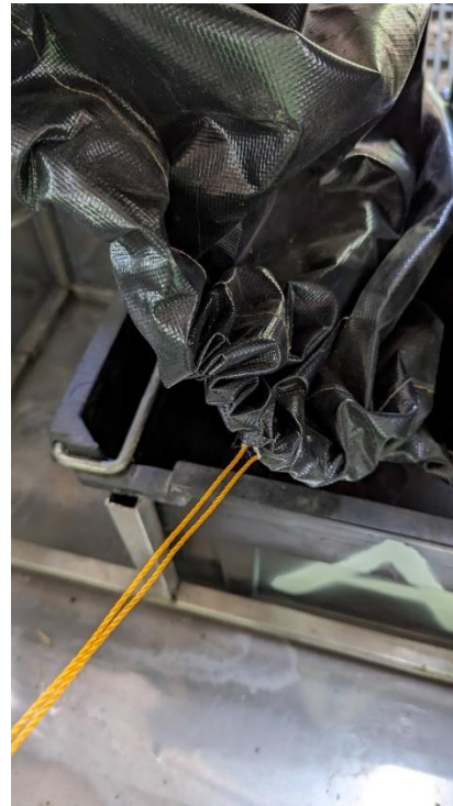
e. Shroud made of vinyl tarpaulin, and its drawcord
