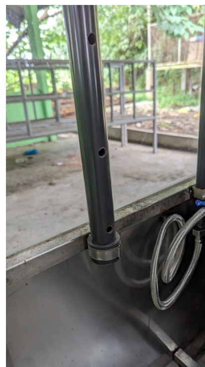
f. Vertical 1-inch pipes with holes for the entry of air to be analyzed
