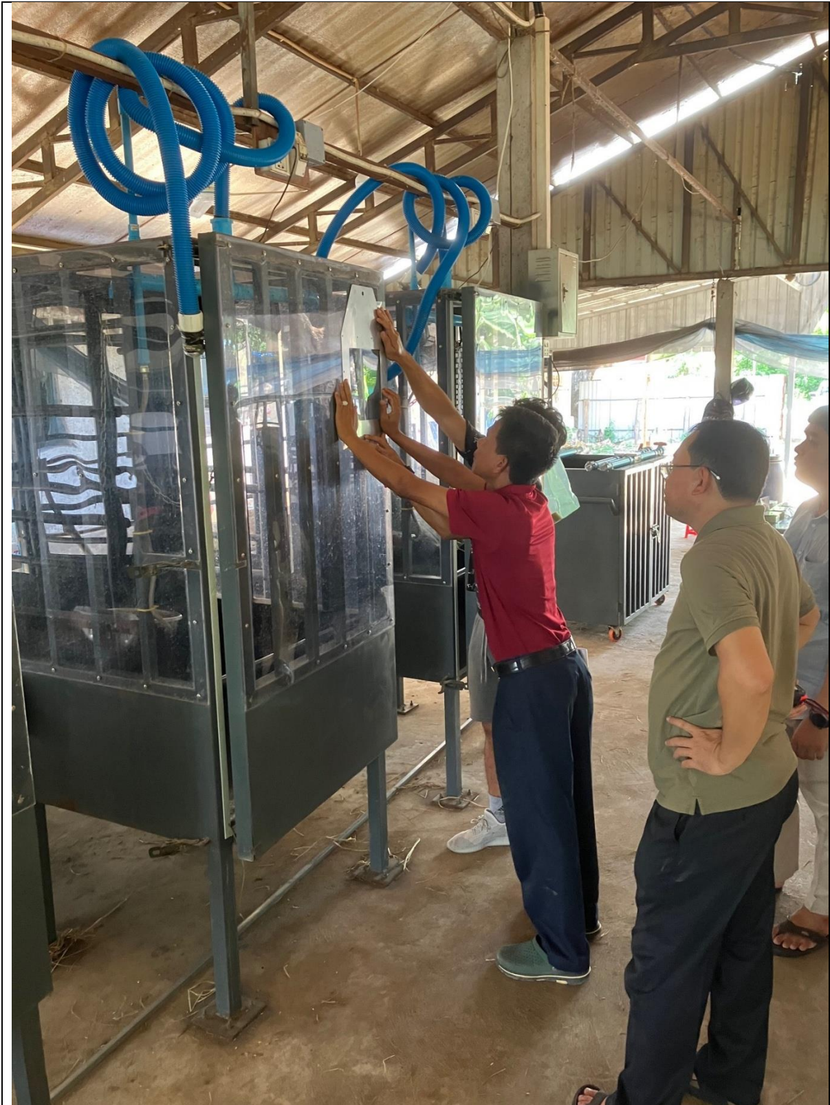
Front view of the chamber showing the blue flexible ducting used to connect the exhaust port (top centre of headbox) to the analysis trolley (shown disconnected at right)
