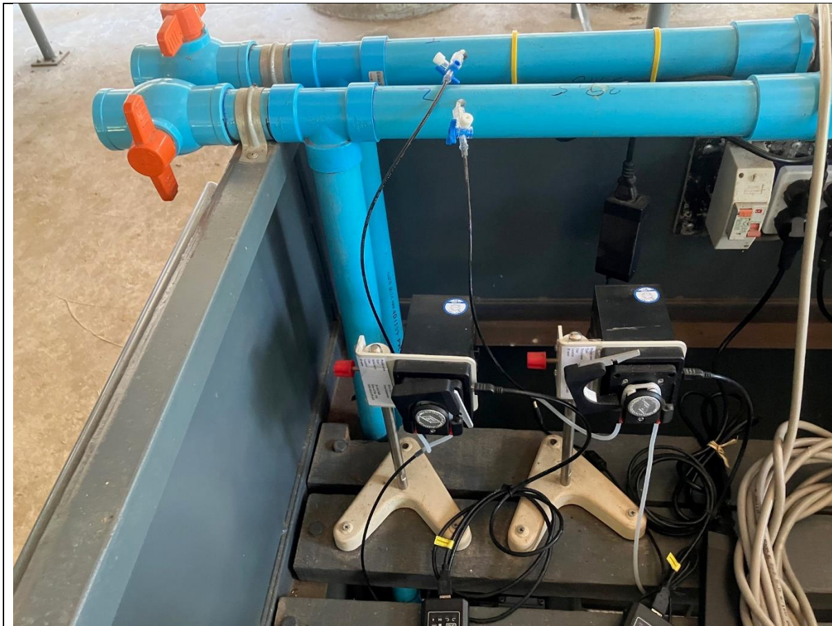
Site of sampling ports in the air flow pipelines. The sampling tubing is connected to the peristaltic pump tube with peristaltic pump collecting 2-2.5 mol/min of air continuously.
