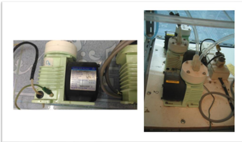
Fig. 8b Vacuum pump for O 2 , CO 2 and CH 4 gas sampling (flow rate 7, 5 and 5 L/min)
