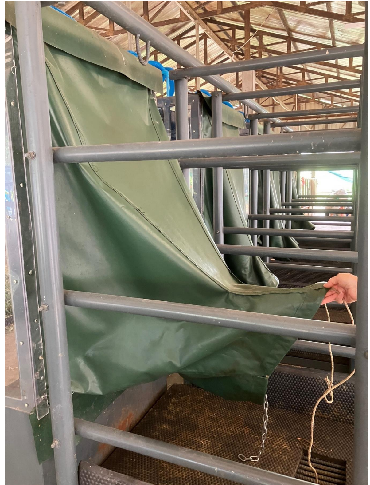
Shroud through which the cow places its head to enter the headbox
