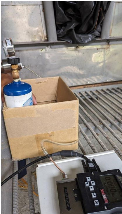
n. Set-up of recovery test wherein the gas is directly infused into one of the inlet pipes.
