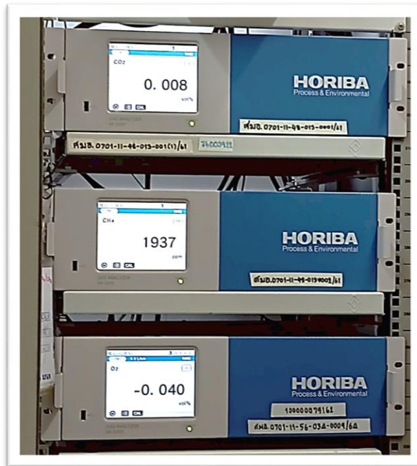
Fig.11 Gas analyzers (Carbon dioxide, Methane and Oxygen)
