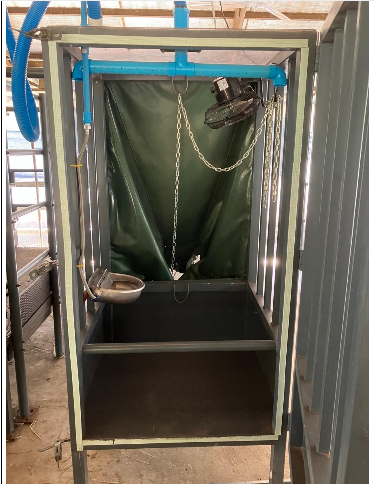
View of the inside of the headbox from the front door. Note bar across front which is used to tether cattle to and chain hanging down that can be used to secure the animal from excessive movement.
