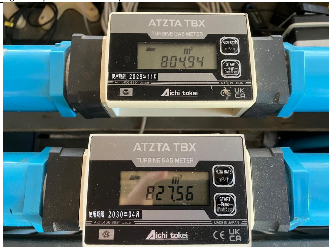
Battery operated turbine flow meters. These can be re-zeroed before each day's study
