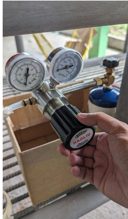
n. Set-up of recovery test wherein the gas is directly infused into one of the inlet pipes.
