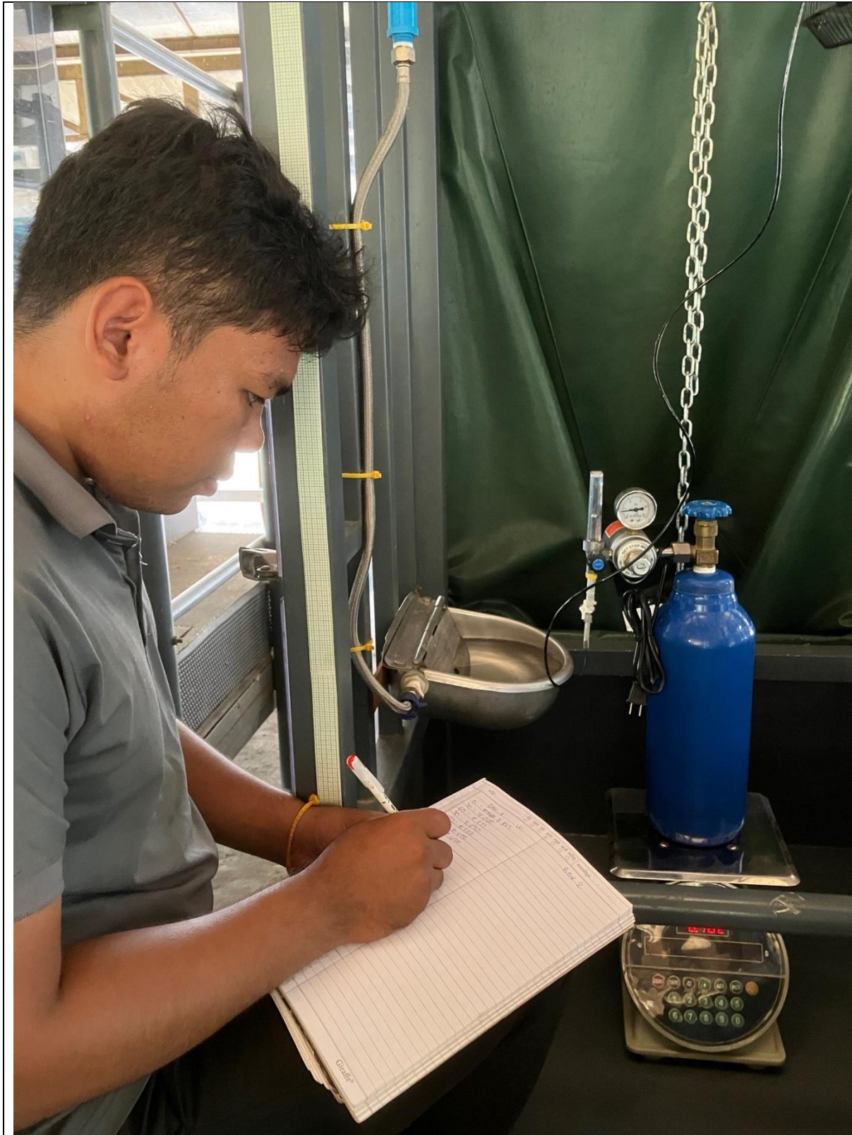
Student reporting the weight of the small CO2 cylinder releasing 5L/min over 3 minutes while also recording the average [CO2] in the airstream leaving the headbox
