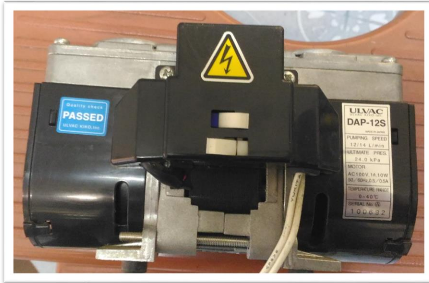
Fig.8a. Pump for air from the main air flow (12 L/min)
